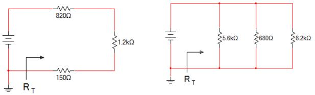
3. Using the laws of circuit theory, solve for R<sub>T</sub>, I<sub>T</sub>, V<sub>R1</sub>, V<sub>R2</sub>, and V<sub>R3</sub>. Be sure to put your answer in proper engineering notation and use the correct units.
